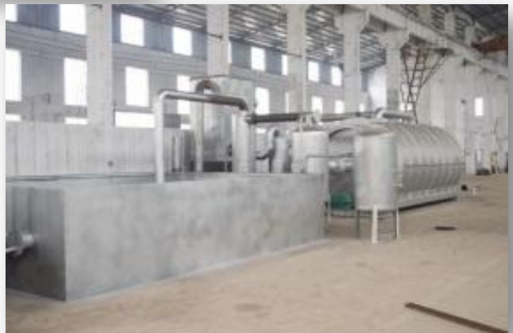
The batch pyrolysis system
